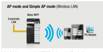
Up to 5 devices can access bizhub 558/458 simultaneously in AP mode with optional UK-212 equipped.
